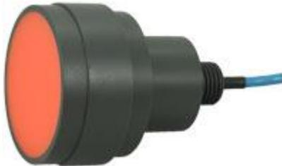
Recent tests of the ETS50200 (Dual channel 50 and 200 kHz transducer), to define how much pressure the sensor can take when mounted flush to the hull, has shown that the transducer withstood over 11MPa of force, the equivalent of more than 11200 kN/m<sup>2</sup>. This is enough to define that the sensors are ice tolerant, for BV ice classes.
